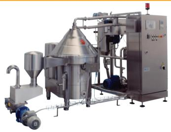
Self-cleaning separator with hydrociclon for fruit juices clarification
