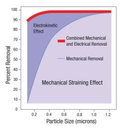
Figure 1: Electrokinetic Effect
