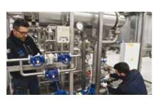
Multi Effect vacuum evaporators Externally heated - energy recycling for minimal operating costs
