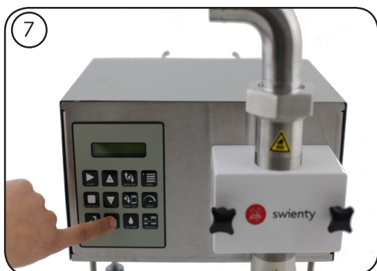
If the dosing amount differs from the real amount, it can be necessary to calibrate more than once.
