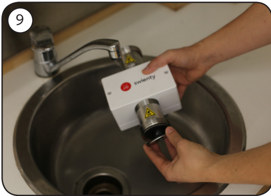
Remove the cutoff mechanism.
