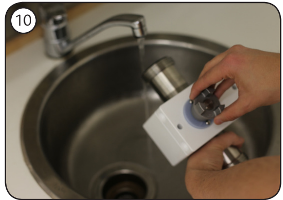
Rinse water through the pump head by turning the clutch. This makes it easier to open the pump head.
