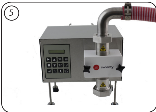
Pump until the air is out of the liquid.
