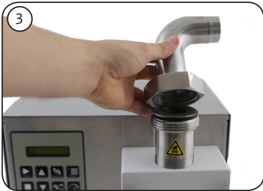
Remove the fitting on top.
