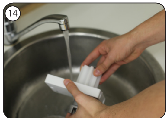
Push slowly on the axis on the cover until a hole appears between the axis and the cover. Rinse here.
