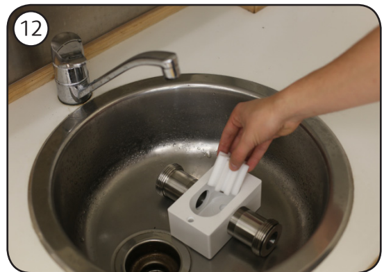
Remove the cog and the axis that is still in the pump head. It can be necessary to rinse with water to loosen it.
