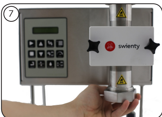
When the machine has stopped dripping, mount the cutoff mechanism. Can be mounted first but not with very viscous liquids. See page 16.
