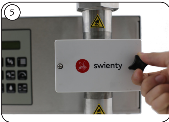
Screw the black nuts off the pump head.
