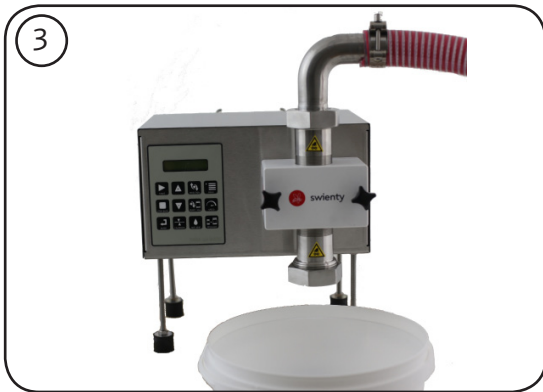
Place a big container below the pump head.
