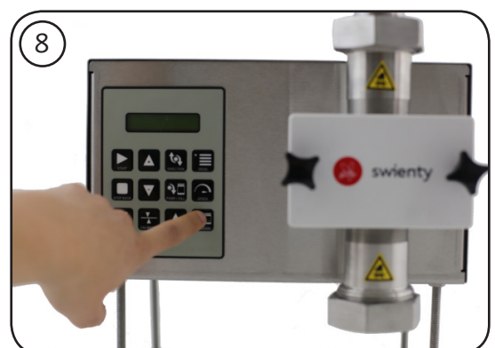
Choose the program that comes closest to the amount you want to dose. Use the button [Progr.].
