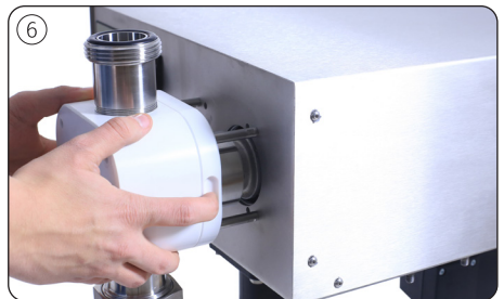
Grasp the notches at the end of the pump housing and gently pull the pump housing off the machine.
