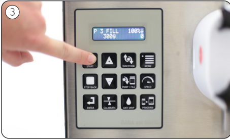
The machine must be set to FILL and the desired program. Press [START] or use the foot pedal.
