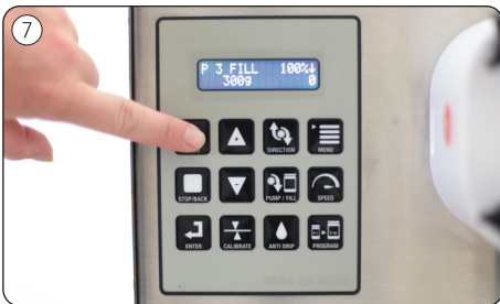
Potentially repeat the calibration if the difference between weight and filling amount is big.
