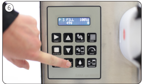
Press [+] and/or [-] until the same number appears on the display. Save by pressing [CALIBRATE].
