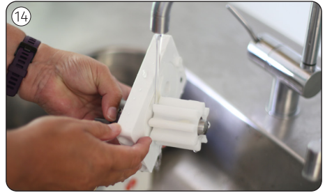
Carefully press on the fixed axis so that a gap appears between the gear and the cover. Rinse here.
