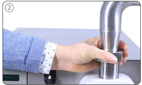
Loosen the connection fitting so air can come into the pump housing, but not so much that the honey starts running out. WARNING: Always disconnect the machine from the power supply before taking the pump apart.
